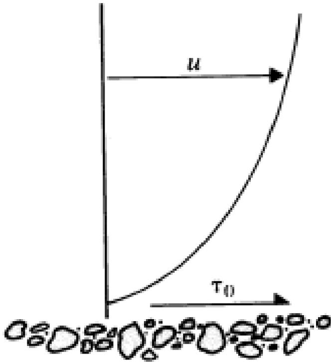
**(a) Shear force on granular bed**
