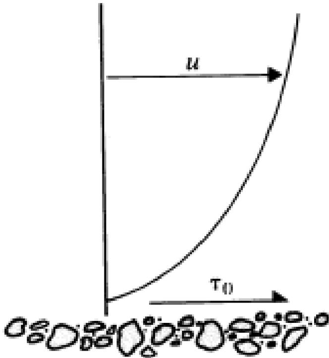
**(a) Shear force on granular bed**
